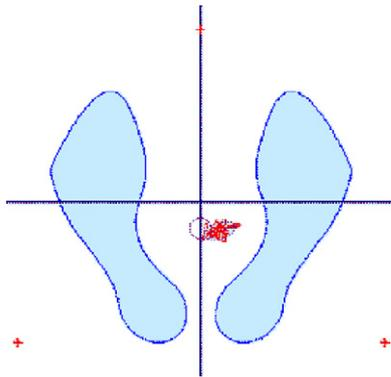
Fig. 1. Reference position given by SATEL<sup>®</sup> and a sample statokinesigram (sway-path measurement).
